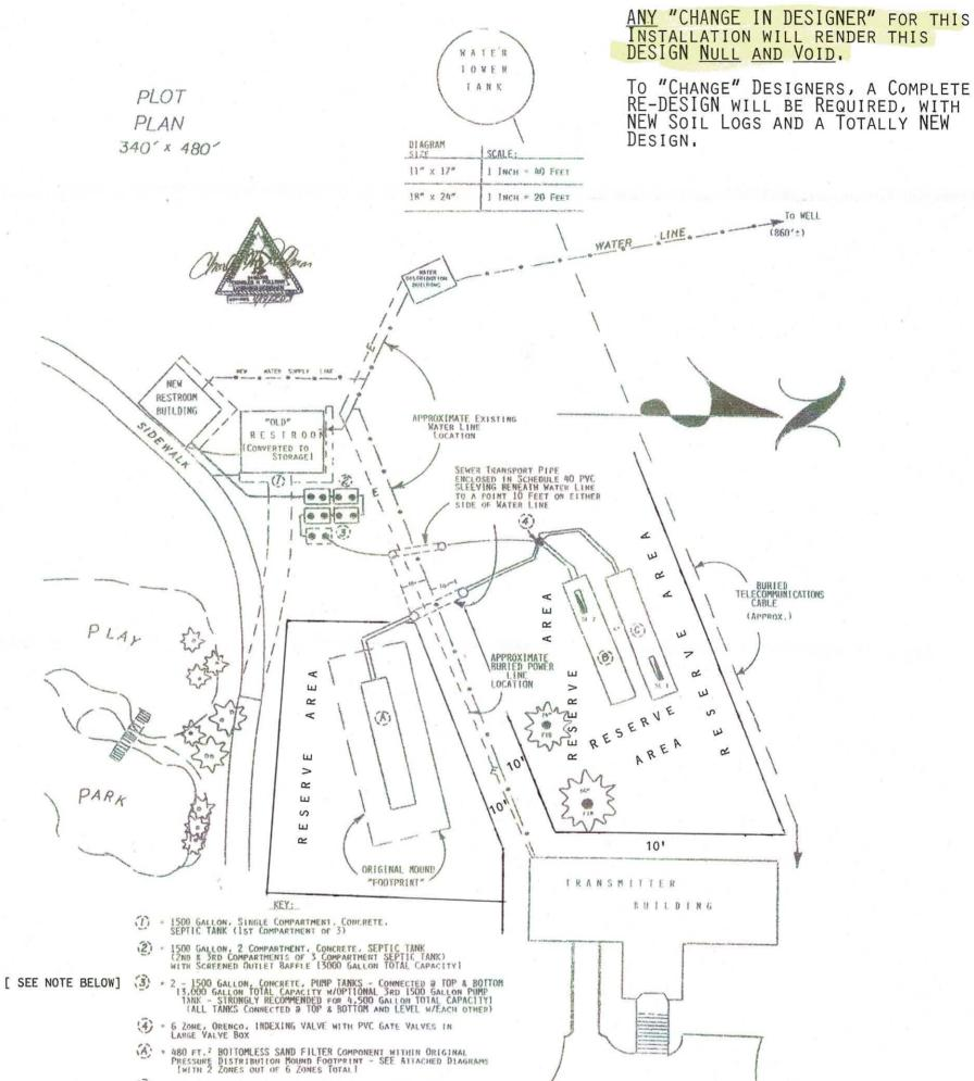
(B) = 480 FT.<sup>7</sup> ROITOMLESS SAND FILTER COMPONENT (10'X 48') EXCAVATED THROUGH COMPACTED TOPSOILS TWITH 2 ZONES OUT OF 6 ZONES TOTAL)
